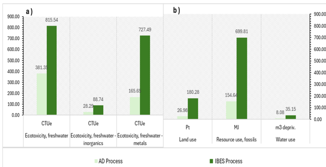
Figure 3.7: Comparative environmental impacts of the AD and IBES processes: (a) ecotoxicity indicators including freshwater ecotoxicity, ecotoxicity from inorganics, and ecotoxicity from metals (measured in CTUe); (b) land use (Pt), fossil resource use (MJ), and water use ( m^3 deprivation). The IBES process shows significantly higher impacts across all categories compared to the AD process
