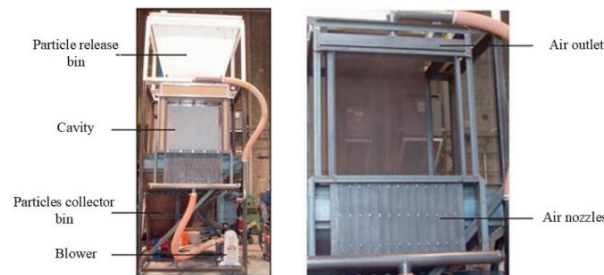
Figure 16 Free-falling solid particle receiver with an air curtain [60]
