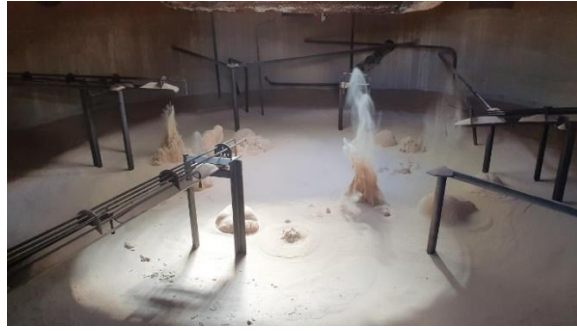
Figure 20 Fluidized sand bed in fluidization process
