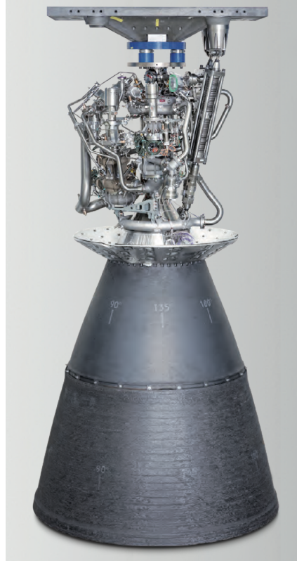
Figure 2.12: VINCI engine foreseen for Ariane 6 upper-stage applications [36]
