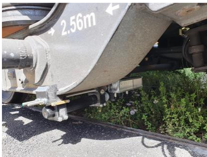
Figure 50 left image: sensor system mounted on the bogie frame; right image: PC for image acquisition and processing, positioned in the coach.
