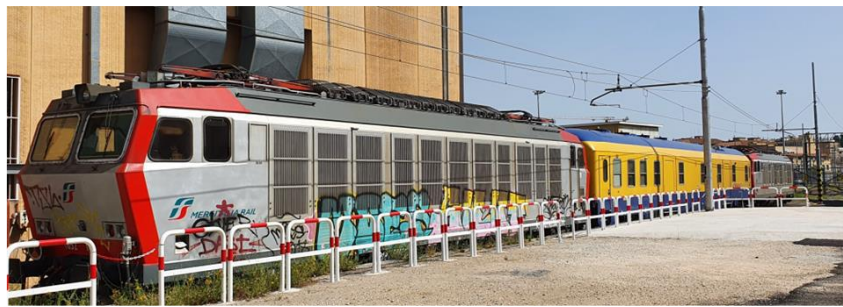
Figure 49 train used for validation test, consisting of two E652 locomotives (leading and trailing) and the Aldebaran 2.0 track recording car.
