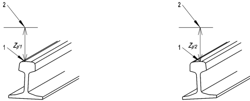
Figure 8 Longitudinal level (SS-EN 13848-1: 2004+A1 2008).
