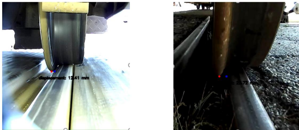
Figure 46 Real-time lateral displacement measurement of the wheel on the rail to support track geometry monitoring (screenshot from the demo videos https://youtu.be/it21cE87LCM and https://youtu.be/Nc1bkQdkkSM )
