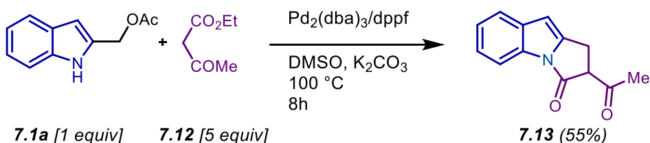
Scheme 7.5. Reaction of 7.1a with ethyl malonate 7.10 and the ethyl-3-oxobutanoate 7.12.
