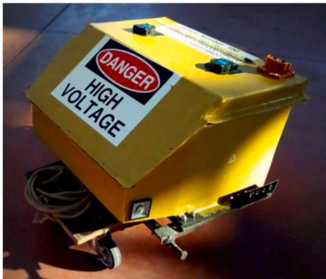
Fig. 4. Battery Pack installed on the vehicle.
