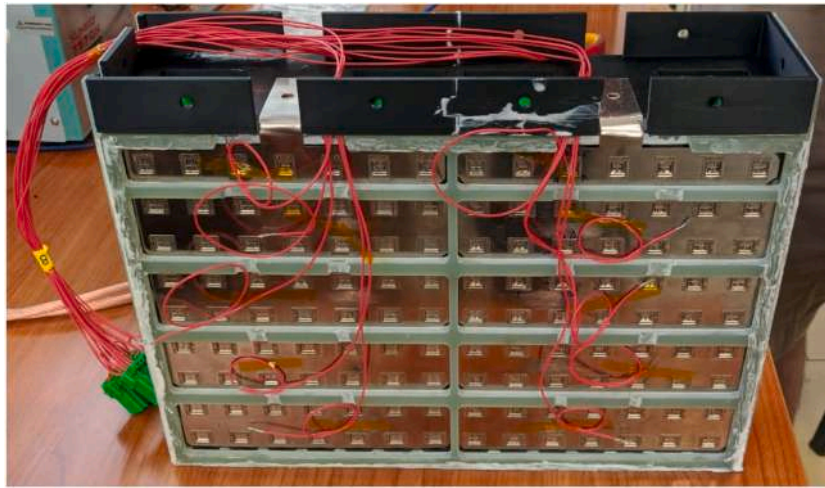
Fig. 15. Forced air-cooled module, 2022 season car.
