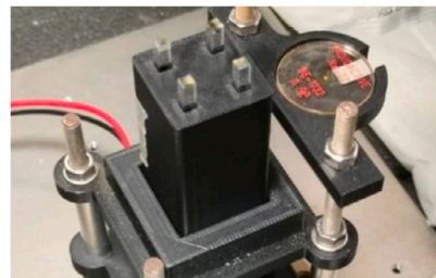
Fig. 1. Picture of the multianode PMT, kept in a 3D printed holder, with four LYSO crystals and the Na-22 source.
