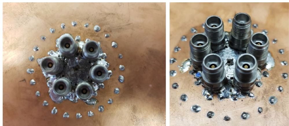
Figure 16. The feeding network realized through a circular array of N = 6 coaxial cables. Two concentric via-hole rings are inserted to enhance the broadband impedance matching. Reproduced from [47].
