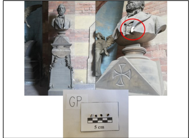
Fig. 2. Bust on pillar funerary monument (sample GP) with the indication of the area (red circle) from which the collected black crusts were detached.
