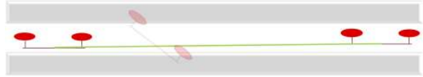
Fig. 2: Due to underactuation, the collision-free path requiring the quadrotor to move with a fixed orientation along the narrow passage is not feasible: frame bending is required to obtain a non-null component of the thrust along the planned path (transparent UAV).
