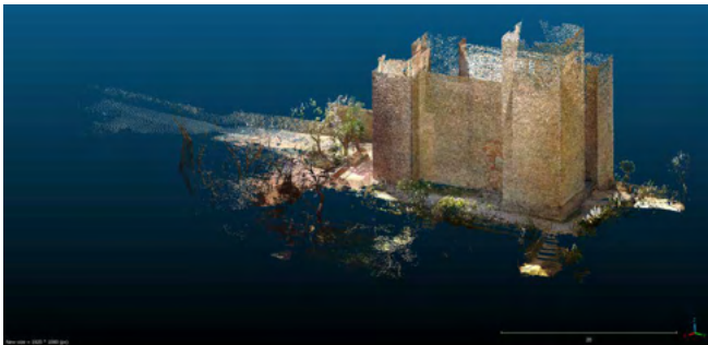
8.7/ Point cloud of Talamone Fortress, generated by eight laser scanner acquisitions.
