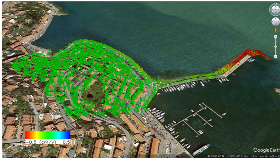
6.10/ Three-dimensional point clouds in Google Earth™ environment, obtained by processing 160 COSMOSkyMed radar images with DEM data from the TanDEM-X mission. Porto Santo Stefano site. Source: Agenzia Spaziale Italiana, 2022. Products processed by Luca Martelli, Diego Reale, and Simona Verde under a license of the Italian Space Agency (ASI); Original COSMO-SkyMed Products - ©ASI - (2012-2017); Deutsches Zentrum für Luft- und Raumfahrt e.V., 2006. © DLR <2023>. Google™ and Google Earth™ are trademarks of Google LLC and this thesis is not endorsed by or affiliated with Google in any way.
