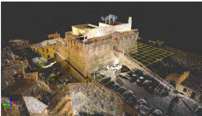
7.4/ Alignment of the first 48 point clouds from laser scanners in the JRC Reconstructor environment. Representation of the Fortress as seen from the north-east.
