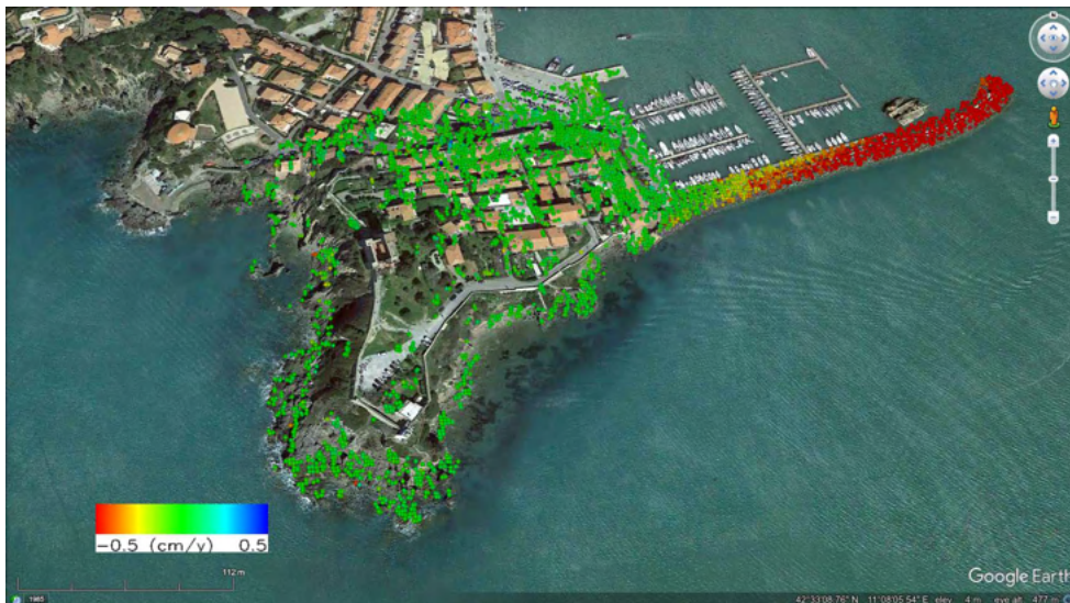
6.11/ Three-dimensional point clouds in Google Earth™ environment, obtained by processing 160 COSMOSkyMed radar images with DEM data from the TanDEM-X mission. Talamone site. Source: Agenzia Spaziale Italiana, 2022. Products processed by Luca Martelli, Diego Reale, and Simona Verde under a license of the Italian Space Agency (ASI); Original COSMO-SkyMed Products - ©ASI - (2012-2017); Deutsches Zentrum für Luft- und Raumfahrt e.V., 2006. © DLR <2023>. Google™ and Google Earth™ are trademarks of Google LLC and this thesis is not endorsed by or affiliated with Google in any way.
