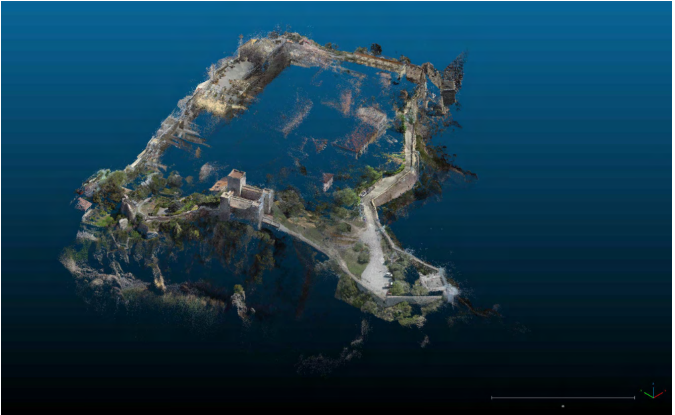
8.11/ Dense cloud of the walls of Talamone and the Aldobrandeschi Fortress, obtained by means of Structure from Motion (SfM) photomodeling in 3DFlow Zephyr environment. Source: Agenzia Spaziale Italiana, 2022. Products processed by Luca Martelli, Diego Reale, and Simona Verde under a license of the Italian Space Agency (ASI); Original COSMO-SkyMed Products - ©ASI - (2012-2017); Deutsches Zentrum für Luft- und Raumfahrt e.V., 2006. © DLR <2023>. Ministero dell'Ambiente e dell'Energia – Italian Ministry of Environment and Energy / licensed under CC BY-SA 3.0 IT ( https://creativecommons.org/licenses/by/3.0/it/deed.it ) / Creative Commons – Attribuzione - Condividi allo stesso modo Italia (CC BY-SA 3.0 IT).
