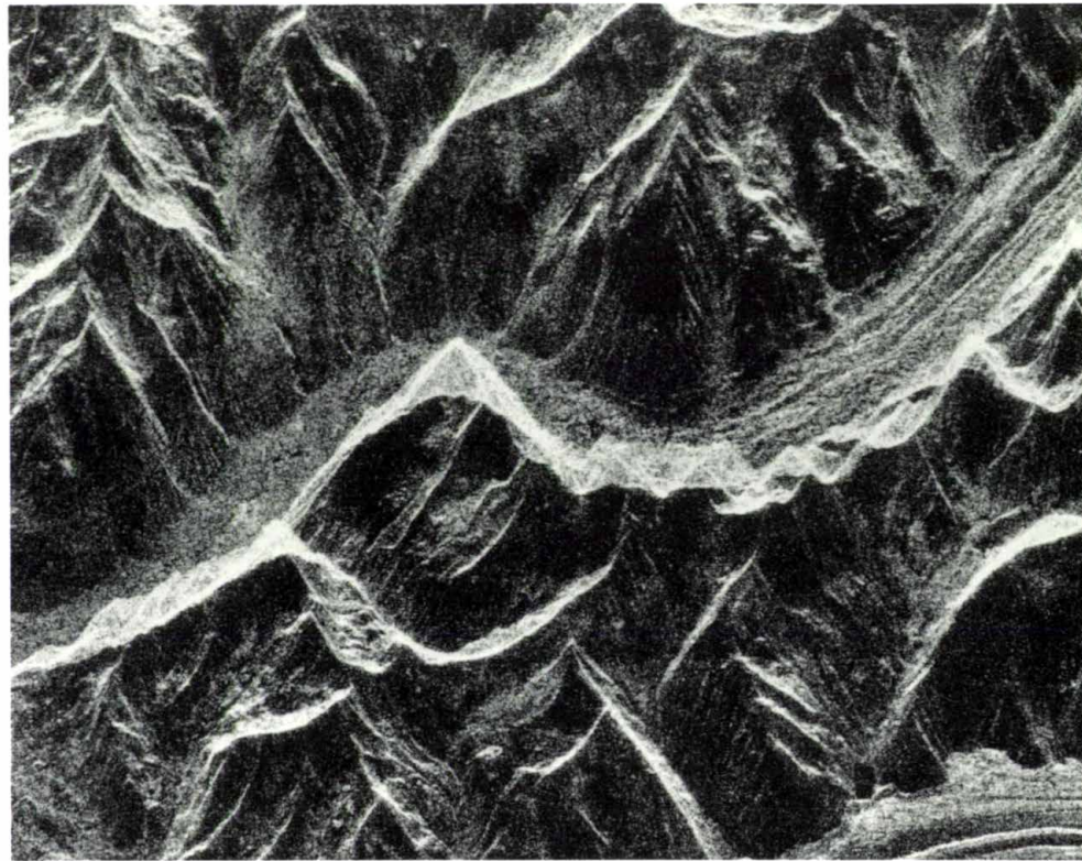
2.12/ Example of layover in a SAR image of the Alaska Range, scanned during the Seasat Mission. Since the sensor was pointing towards the underside of the image and the mountain ranges have a steep slope, this resulted in an layover effect of the mountain top (bottom) on the glacier at its foot (centre of the image). The glacier can be easily identified by the ice tongue on the right. Note the progressive stretching of the radar image as one scrolls from the upper to the lower side. Source: Ford, Blom, Crisp, Elachi, Farr, Saunders, Theilig, Wall, Yewell 1989 / Image under Public Domain.
