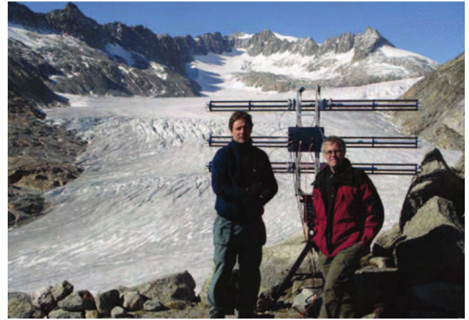
1.19/ A portable Real Aperture Radar (RAR) interferometer in front of the Rhone Glacier in the Valais region of Switzerland. The photo allows an approximate comparison of the size of the instrument with the human scale. Source: Werner, Strozzi, Wiesmann, Wegmüller 2008. © 2008 IEEE.
