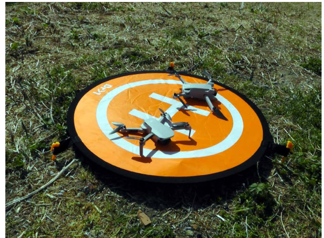
8.8/ Fleet of drones (a Mavic DJ Mini Pro 2 and a Mavic DJ Mini Pro 3) with cameras for the survey of Talamone Town Walls by means of Structure from Motion photomodelling.
