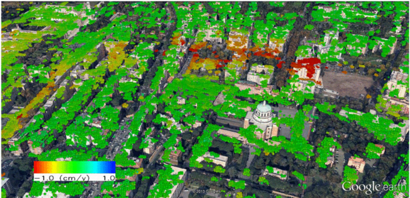
3.24/ Three-dimensional visualisation, in Google Earth™ environment, of the scatterers detected through four-dimensional tomographic processing in the Grotta Perfetta area in Rome, Italy. The colours were set according to the estimated values of average deformation velocity (in cm per year). Source: Fornaro, Pauciullo, Reale, Zhu, Bamler 2012. © 2012 IEEE. Google™ and Google Earth™ are trademarks of Google LLC and this thesis is not endorsed by or affiliated with Google in any way.
