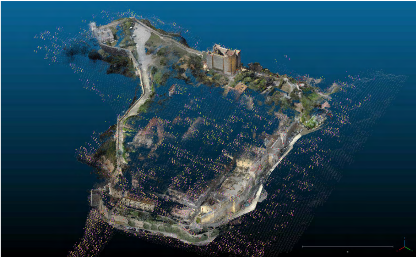
8.10/ Dense cloud of Talamone Town Walls and the Aldobrandeschi Fortress, obtained by means of Structure from Motion photomodelling in the 3DFlow Zephyr environment and superimposed on the supporting composite cloud. The composite cloud consists of: the laser scanner cloud of the Rocca aldobrandesca (coloured); the PST-A cloud of the Italian Ministry of the Environment (white); the tomographic cloud with NASADEM data (yellow); the tomographic cloud with TanDEM-X data (magenta); the topographic cloud obtained through Total Station (red). Source: Agenzia Spaziale Italiana, 2022. Products processed by Luca Martelli, Diego Reale, and Simona Verde under a license of the Italian Space Agency (ASI); Original COSMO-SkyMed Products - ©ASI - (2012-2017); Deutsches Zentrum für Luft- und Raumfahrt e.V., 2006. © DLR <2023>. Ministero dell'Ambiente e dell'Energia – Italian Ministry of Environment and Energy / licensed under CC BY-SA 3.0 IT ( https://creativecommons.org/licenses/by/3.0/it/deed.it ) / Creative Commons – Attribuzione - Condividi allo stesso modo Italia (CC BY-SA 3.0 IT).
