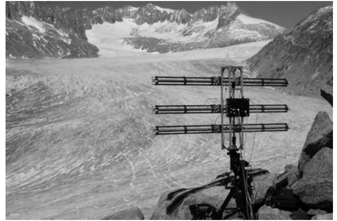
1.15/ Portable Real Aperture Radar (RAR) interferometer during a scan of the Rhone glacier in the Valais region of Switzerland, performed on 6 September 2007. Source: Strozzi, Werner, Wiesmann, Wegmüller, 2012. © 2012 IEEE.
