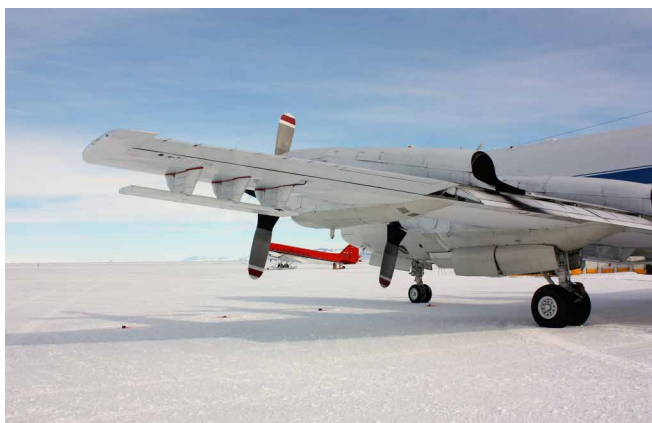
1.26/ One of the radar antenna arrays of the Multichannel Coherent Radar Depth Sounder (MCoRDS), mounted under the wing of NASA's P-3 aircraft. The MCoRDS employs panels under the wings and fuselage of the aircraft, for a total of 15 antennas that can transmit and receive signals in order to map the polar ice and the rock bed below. Source: National Aeronautics and Space Administration, 2013a / Image under Public Domain. Crediti: NASA / George Hale.
