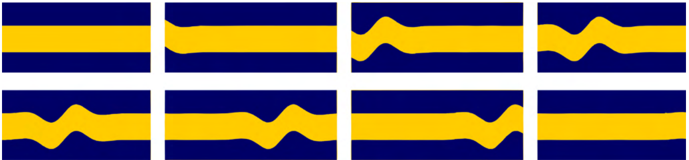
1.3/ Graphical illustration of the behaviour, in time and space, of a transverse wave front travelling through a medium. Source: Gallis 2004.
