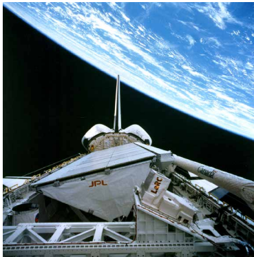
1.21/ Photograph of the Spaceborne Imaging Radar-C/X-Band Synthetic Aperture Radar (SIR-C/X-SAR) sensor at the Jet Propulsion Laboratory. The radar is placed in the payload bay of the orbital space shuttle Endeavour (STS-59). In the background, an area of the Pacific Ocean northeast of Hawaii. The antenna of the SIR-C/X-SAR, consisting of a triangular support structure and flat panels [flat antenna panels], is capable of collecting data within three frequency bands simultaneously: C-band, L-band and X-band. When this picture was taken, in 1994, six NASA astronauts spent a week and a half in Earth orbit in support of the SIR-C/X-SAR mission. Source: National Aeronautics and Space Administration, 1998 / Image under Public Domain. Credits: NASA/JPL.
