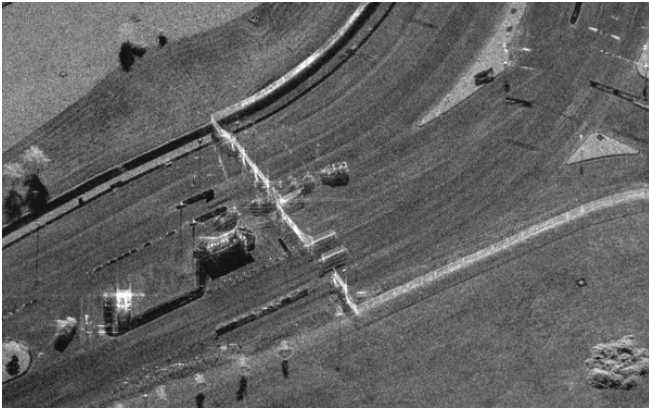
4.2/ Radar image of the barrier at the driveway entrance to Kirtland Air Force Base near Albuquerque, New Mexico, acquired by Sandia National Laboratories using a synthetic aperture sensor operating in Ka-band. Given the image apparent resemblance to a photograph, the lighter pixels, even arranged like four-pointed stars, would suggest a bright reflection, such as that typical of a highly polished metallic object. In reality, bodies with such a strong radar reflection "only" have a geometric configuration and dielectric properties such that they backscatter a large portion of the signal transmitted by the sensor. Source: Sandia National Laboratories, 2023a. Courtesy of Sandia National Laboratories, Radar ISR.
