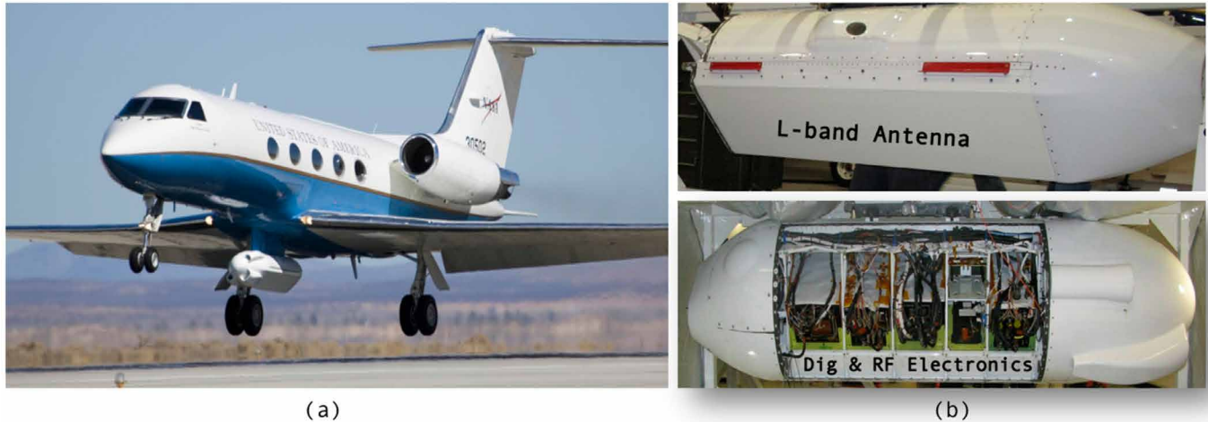
1.20/ Experimental SAR, mounted on aerodyne and operated by pulses at the L frequency band. (a) Aircraft sensor platform, consisting of a Gulfstream-3 jet. The Radar is embedded in a pod located under the fuselage. (b) Details of the pod, with the antenna on the outer surface and the other components inside. Source: Jones, Holt 2018 / licensed under CC BY 4.0 ( http://creativecommons.org/licenses/by/4.0/ ). © 2018 by Jones, Holt. Licensee MDPI, Basel, Switzerland.
