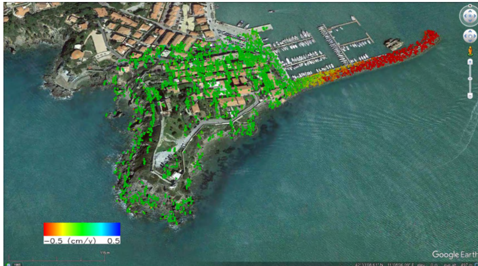
6.7/ Three-dimensional point cloud in Google Earth™ environment, obtained by processing 160 COSMOSkyMed radar images with NASADEM data. Talamone site. Products processed by Luca Martelli, Diego Reale, and Simona Verde under a license of the Italian Space Agency (ASI); Original COSMO-SkyMed Products - ©ASI - (2012-2017); Google™ and Google Earth™ are trademarks of Google LLC and this thesis is not endorsed by or affiliated with Google in any way; United States Geological Survey, National Aeronautics and Space Administration 2020.
