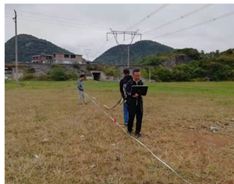
Fig. 12 Photograph shows GPR acquisition on grass land under high voltage lines
