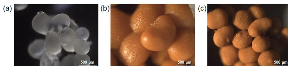
Figure 4. Optical microscopy images of dried (a) Alg, (b) Alg/Z5A/Cur, and (c) Alg/Z5A/Cur/CS beads.
