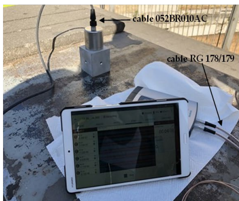
Figure 4. Instrumentation of the experimental setups: (a) acquisition system (LMS SCADAS XS and LMS Smart Scope), (b) LMS SCADAS XS, (c) piezoelectric accelerometer (model 393B31), (d) and (e) connections views
