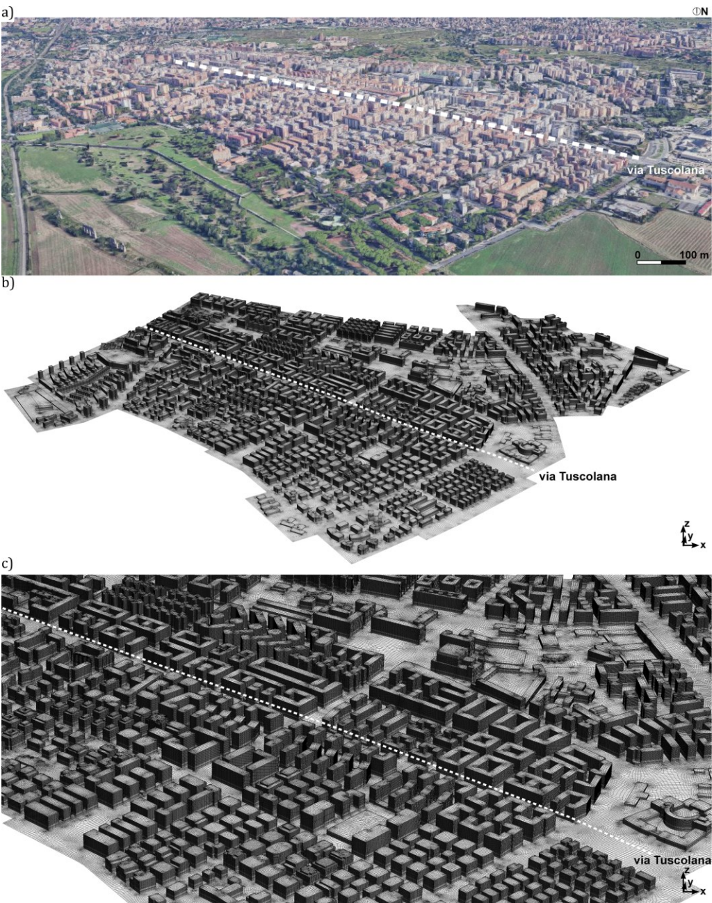
Fig. IV 6 - Perspective view of: (a) the area of interest (modified from Google Maps); (b) the computational grid and (c) its enlargement. The total cell count is about 86 million.
