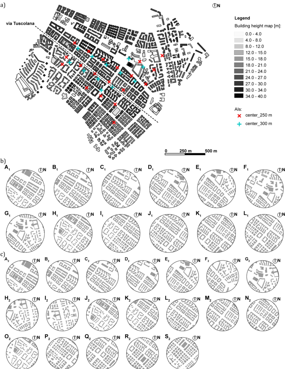
Fig. IV_2 - (a) Map of the height [m] of the buildings modeled in the domain with the locations of the center of the AIs; plan view of the 31 AIs considered in the study with (b) 300 m radius and (c) 250 m radius.
