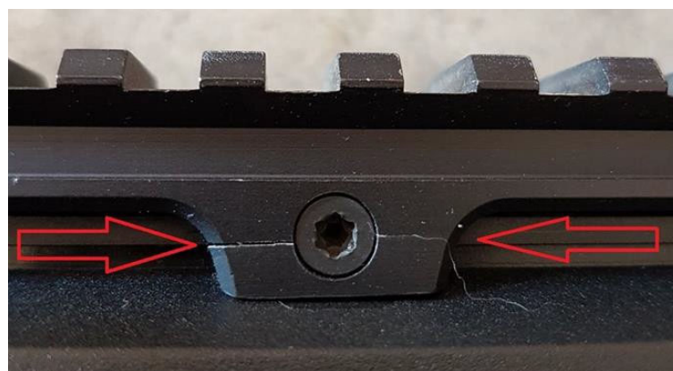
Figure 14 - example of technical inconvenience: mechanical damage in the rail of automatic rifle.
