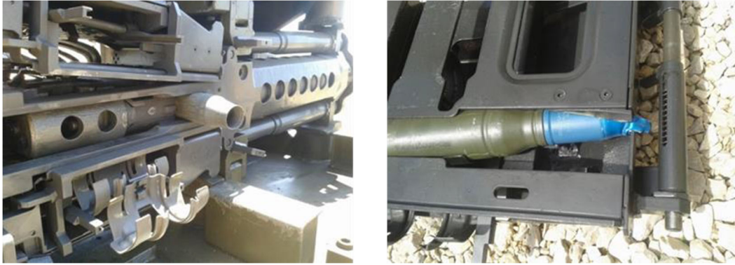
Figure 15 - example of a technical inconvenience for cal. 25 mm machine gun: jammed munitions
