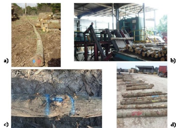
Figure 3 - a) curvature of the lumber, b) trimmer machine, c) chestnut canker where the bole is eliminated, d) chestnut lumber
