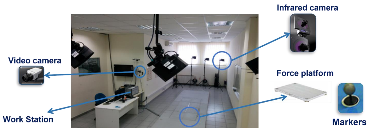
Figure 3.3 Components of SMART system.
