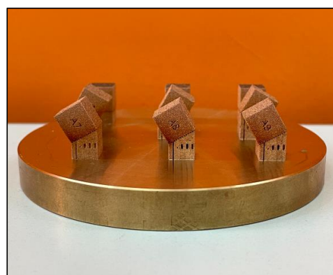
Figure 3. Print Job I: A# specimens' production results on the building platform.
