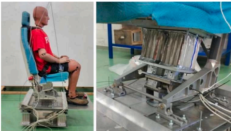
Fig. 12. Aluminum honeycomb energy absorber under a rotorcraft seat [136]. The image to the right is a zoom section of the aluminum honeycomb.
