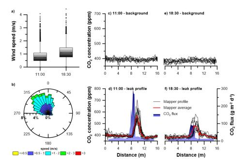
**Figure 4.** Data from sensitivity tests at the Bassano controlled release site on 18/9/20: a) wind speed distribution during the two measurement periods; b) wind direction during both periods; Mapper profiles outside (c, e) and across (d, f) the leakage plot at around 11:00 and 18:30, respectively. Note all profiles were performed at a survey speed of about 2.5 km hr<sup>-1</sup>.
