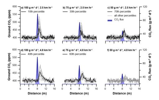
**Figure 5.** Simulations of the Mapper response while traversing a synthetic, 2 m-wide, symmetrically distributed leakage area, taking into consideration system noise. Two different survey speeds and three different maximum flux rates are shown (see legends). Grey lines represent Mapper simulation results while the thick black lines highlight the "first" simulation (i.e., lowest input percentile) that clearly defines the anomaly (see text for details).
