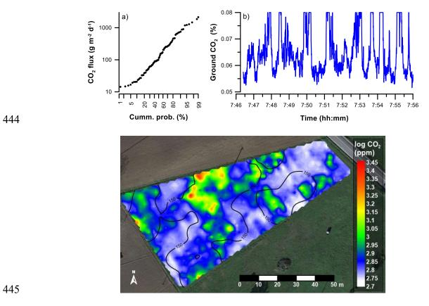
**Figure 7.** Additional plots of the Ailano field data: (a) cumulative probability plot of the flux dataset; (b) representative 10 minutes of the Mapper data from the NE end of Figure 6c, plotted with a 2 point running average and truncated at 800 ppm to highlight lower concentration trends; and (c) same as Figure 6c but plotted as a logarithmic scale of ppm values (150 g m<sup>-2</sup> d<sup>-1</sup> CO<sub>2</sub> flux contour from Figure 6b given for spatial reference).
