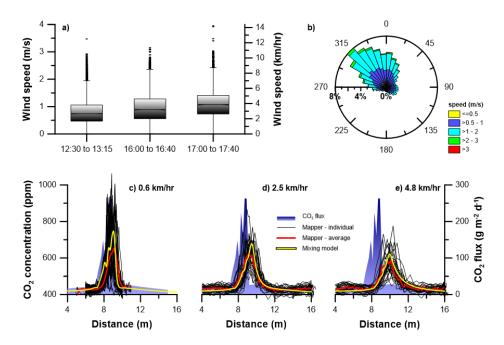
Figure 3. Data from reproducibility tests at the Bassano controlled release site on 17/9/20: a) wind speed distribution during the three measurement periods; b) wind direction during all test periods; c) − e) 30 Mapper replicates (2-point running average) and associated total average for three different survey speeds, together with modelled Mapper response based on the median ground CO₂ concentrations calculated using the shown flux distribution and Eqn.
