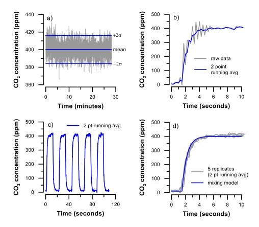
**Figure 1.** Laboratory data illustrating the Mapper response characteristics, including: (a) system noise; (b) saw-tooth trend during a rapid concentration change; (c) response time and reproducibility; and (d) modelling of the system response relative to the data in (c).
