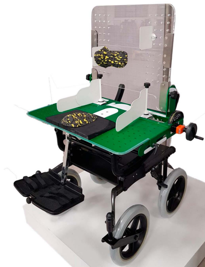
Figure 1. Experimental device used for x-ray examination. The experimental device is considered an evaluation tool for simulating different postural configurations. In fact, it presents easily adjustable parameters for anthropometric measures and applying different postural components and supports is possible. Over the seat and the back, it is possible to apply a customized seating system or a commercial one.
