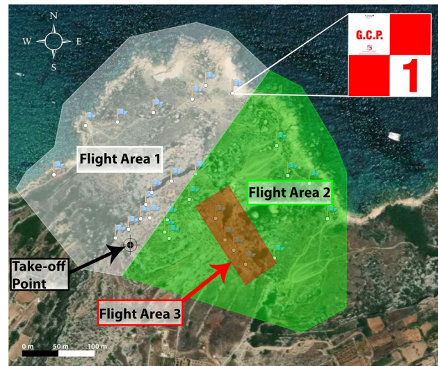
Fig. 2 Satellite image (Retrieved from https://planet.openstreetmap.org ) of the Selmun promontory showing areas of the two flight plans in autonomous mode (flight 1 white area and flight 2 green area) and area 3 (in red) detected in manual flight mode 15 m from the target surface. The take-off point is indicated by a black crosshair and the locations of the Ground Control Points (detailed in the upper right corner) are represented by the blue flags
