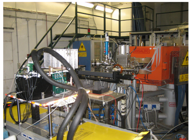
Fig. 16. Experimental setup of the Proto-16 test at the LNF Beam Test Facility (BTF). The beam comes from the right. On the left, the detector inside its case (black) is placed on a movable table to allow for centering of the calorimeter with respect to the beam. In front of the calorimeter, a plastic scintillator bar wrapped in black Tedlar is used to determine the arrival time of the beam electrons.
