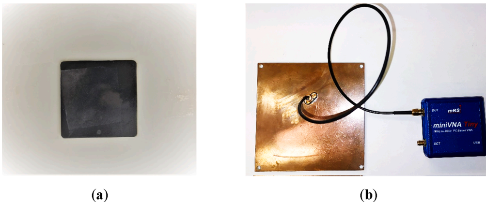
Fig. 2. Proposed system. (a) Patch resonator with the electrically conductive silicon layer; (b) probe and miniVNA-Tiny.
