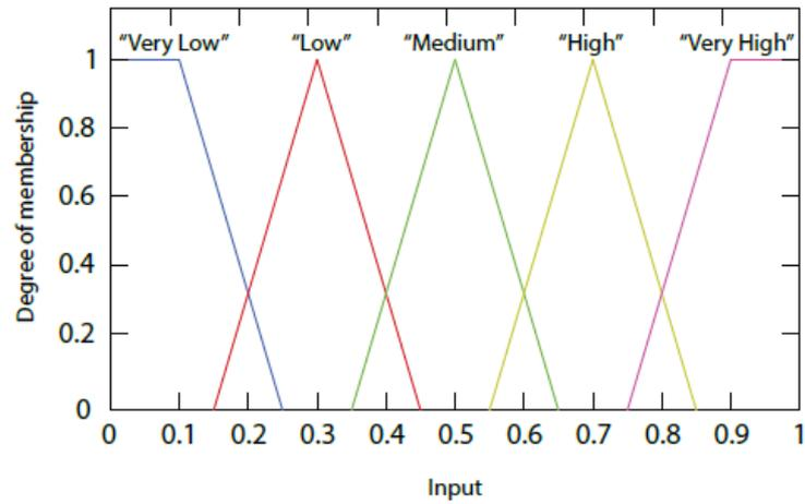
Figure 26. The Term Set for EMS inputs and outputs.
