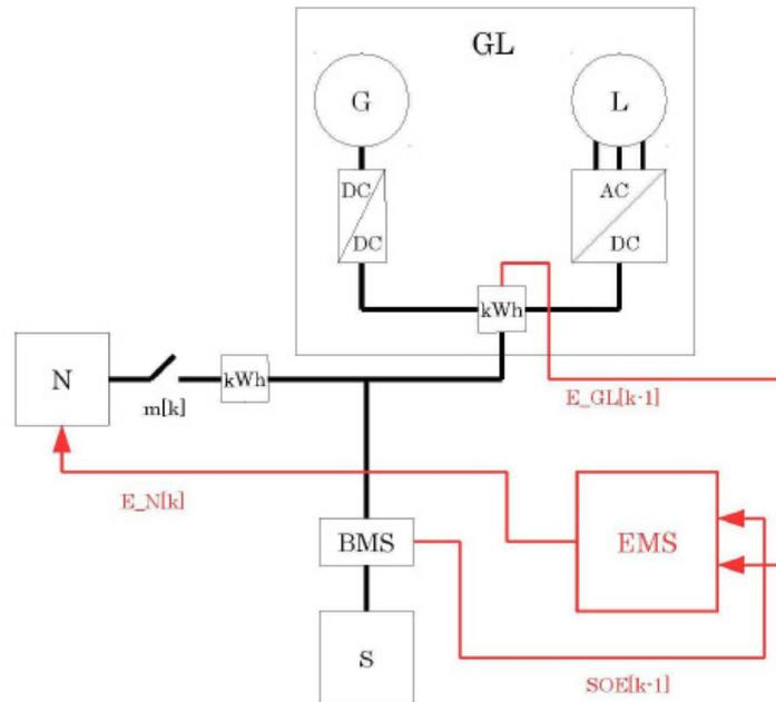
Figure 4.4 - The e-boat MG architecture.
