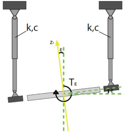
Figure 4.2 - ISWEC linear damper model.
