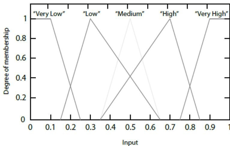
Figure 4.6. Universe of Discourse coverage after deleting a MF (in this case, the central one).
