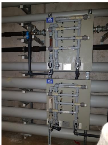
Fig 41: Contact chambers between ACS and specimens
