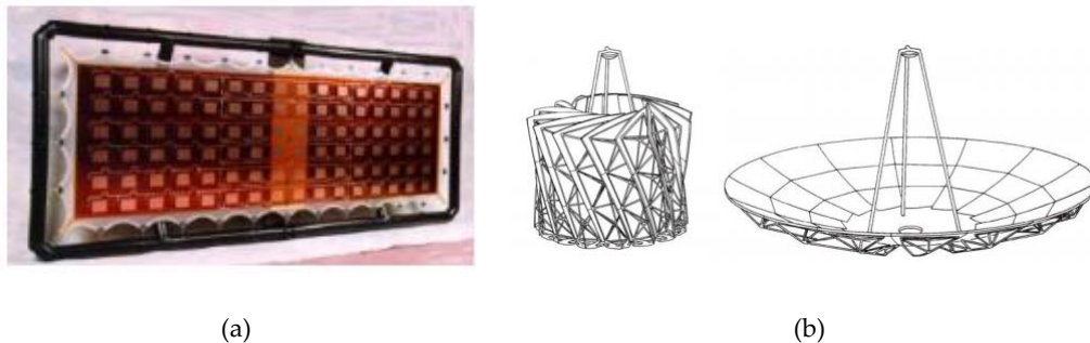
Fig. 2-6: (a) Inflatable membrane antenna [19] (b) DAISY antenna: folded and deployed configurations [21]
