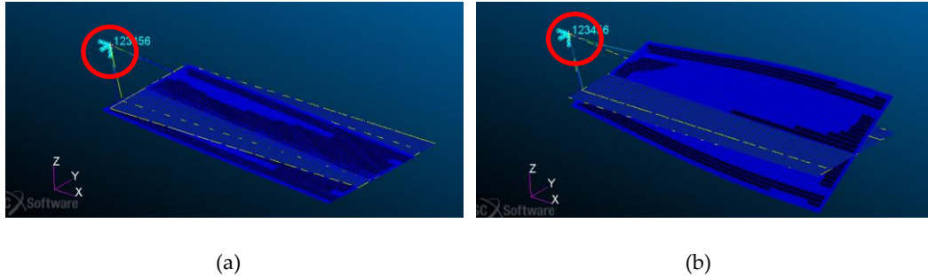
Fig. 5-55: (a) Modal Energy Strain extracted from Nastran (1 st mode); (b) Modal Energy Strain extracted from Nastran (3 rd mode)
