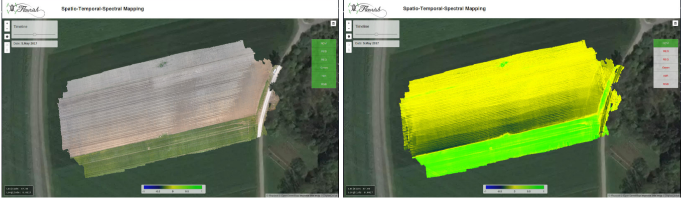
Fig. 9. Visualization interface for the spatio-temporal-spectral database showing both RGB orthomosaics (left) and corresponding index maps (right) for a sugar beet field over time. The user can select spectral layers to view a georeferenced reflectance orthomosaic corresponding to a wavelength band, view the color orthomosaic, and toggle through all available surveys using the timeline.
