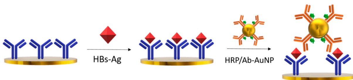
Figure 4. HBV sensor for the detection of HBsAg with HRP/Ab-AuNPs.
