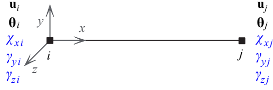
Figure 3: Standard (black) and warping (blue) nodal DOFs for the EVDE model
