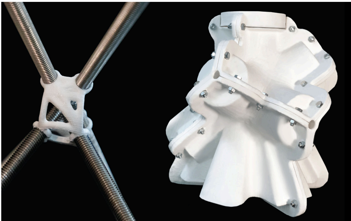
Figure 4. a) 3D printed fixture for an accurate welding process of the threaded rods which are placed within the node; b) 3D printed mould for a 6-axis node consisting of five assembled sub-parts which assure ease in demoulding process.
