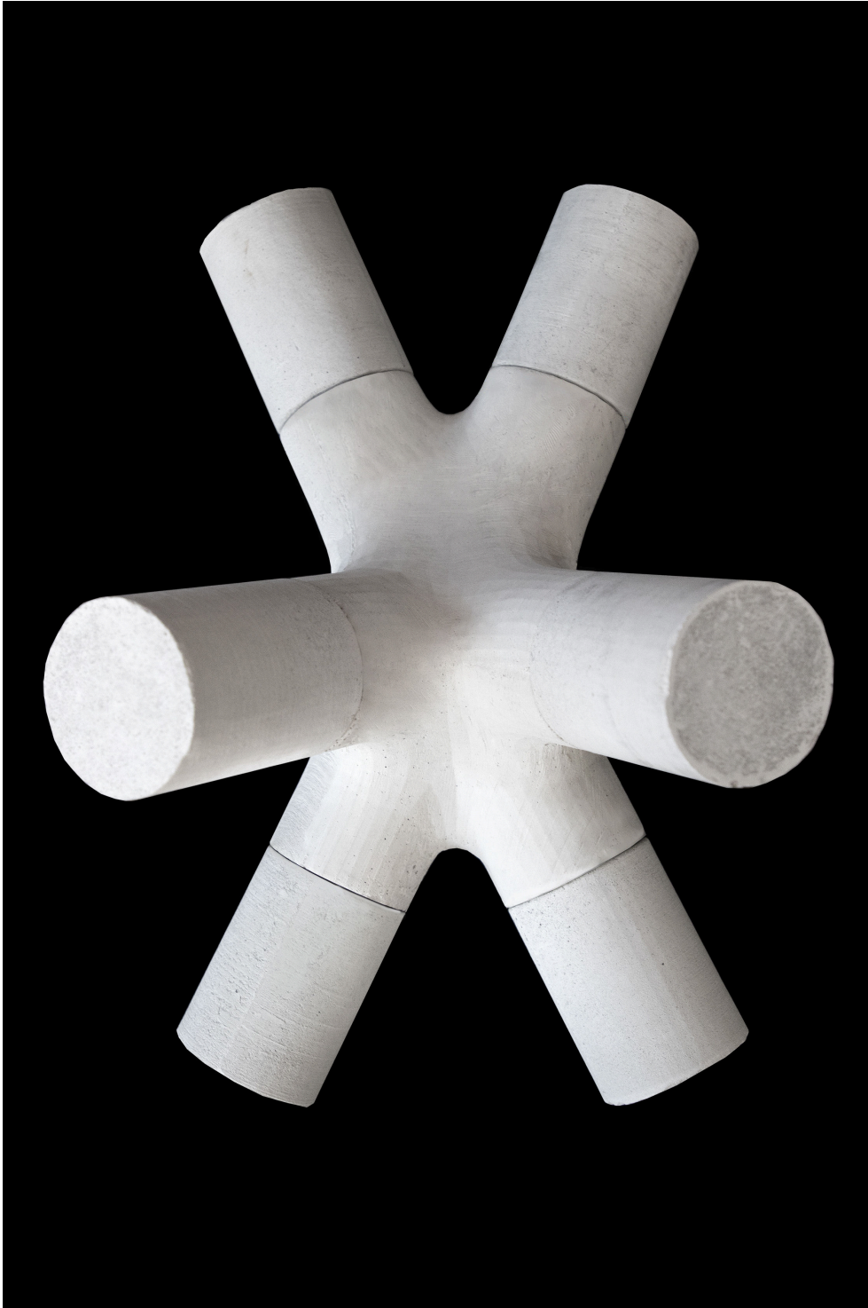
Figure 5. An assembly of a 6-axis node and the complementary struts.
