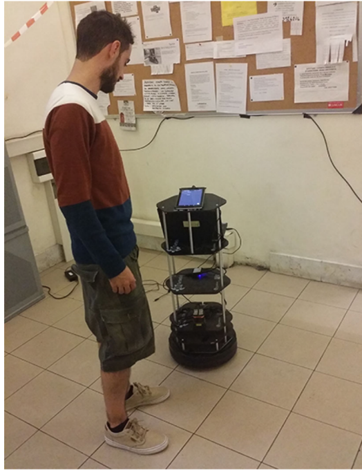
Figure 49. Modified Turtlebot robot. The platform deployed is higher than the standard version, and features a tablet which is used to carry out interactions with users.
