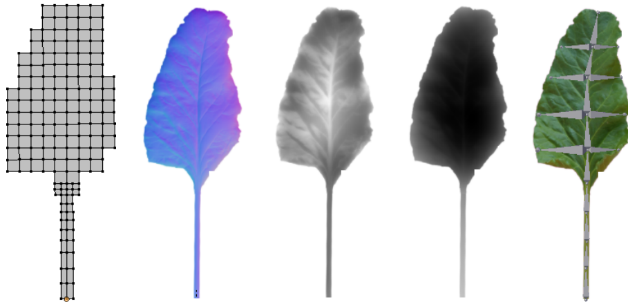
Figure 2.7. (a) Shows the generic planar surface mesh. The number of polygons' subdivisions can be kept as low as possible at the expense of deformation quality while acting on the skeleton. (b) Highlights the Normal Map while (c) and (d) respectively represent the Ambient Occlusion and the Heightmap. (e) Shows the final shading results as well as the skeleton.
