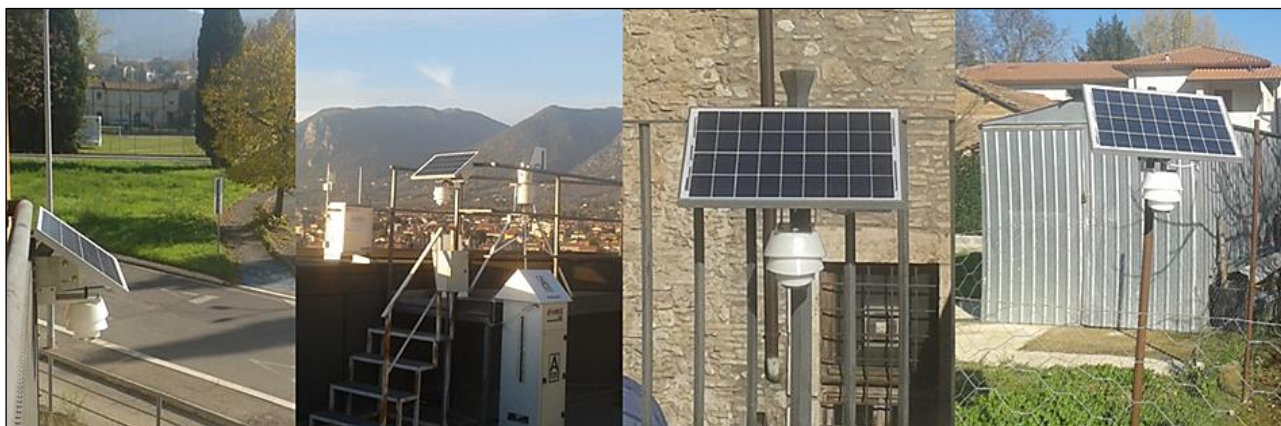
Fig. 2. Smart samplers (SMART SAMPLER Fai Instruments, Fonte Nuova, Roma, Italy) installed in 4 of the 23 monitoring sites of Terni.
