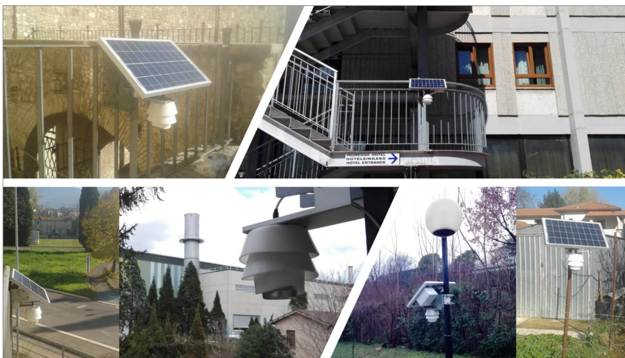
Fig.1. Samplers (HSRS - High Spatial Resolution Sampler; Fai Instruments, Fonte Nuova, Rome, Italy) deployed in Terni.
