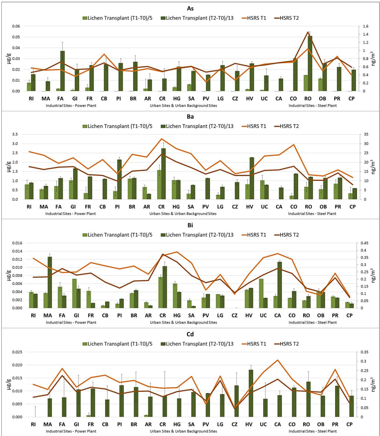
Fig. S3.1. Comparison of As, Ba, Bi and Cd accumulation in lichen samples after five months (T1) and thirteen months (T2) of exposure with their mean concentrations measured in PM 10 during five (HSRS T1) and thirteen (HSRS T2) months.
