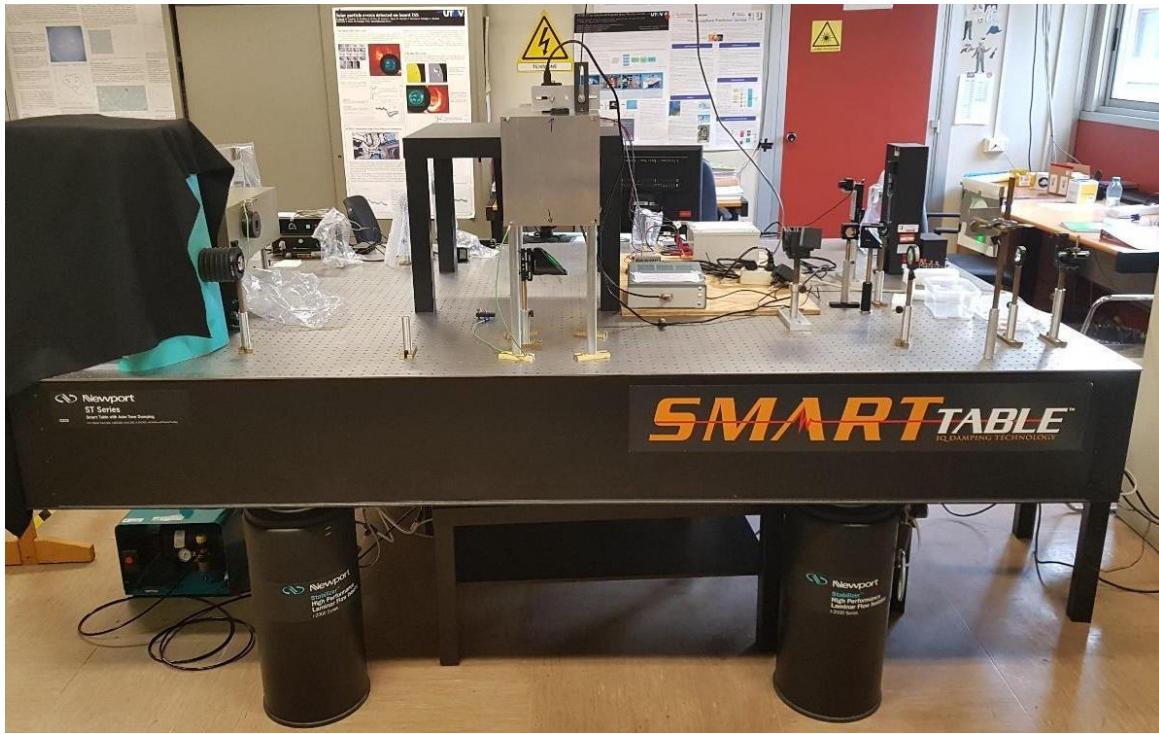
Figure 3.18: Newport Smart Table ST series optical table with the optics for the test. On the left: Sodium lamp with optics for collimated beam. At the center: GREST FPI 50 prototype on four perches with the 45° inclined mirror. On the right: green laser with optics for the collimated beam.
