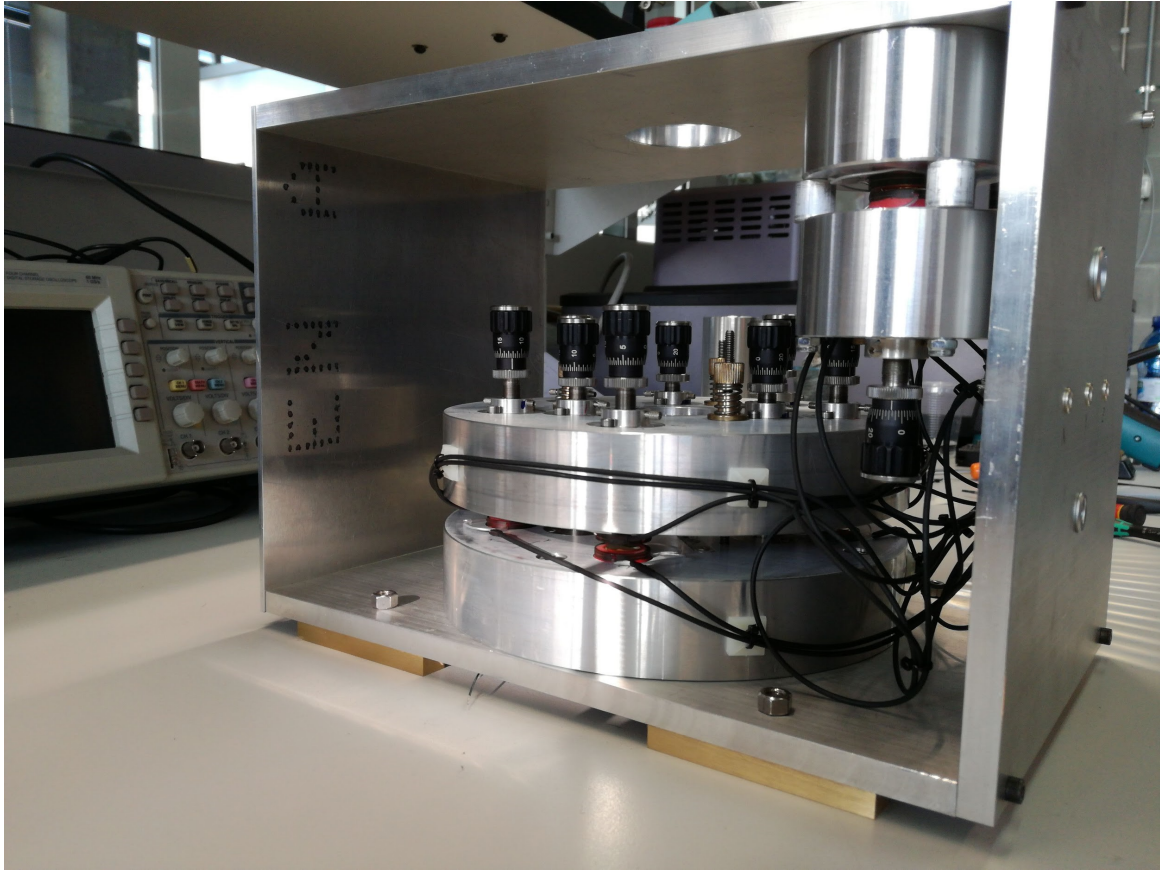
Figure 3.14: Lateral view of the GREST FPI 50 integrated with DM10 micrometers and placed in the housing. All cables are fixed in position during the assembly phase.
