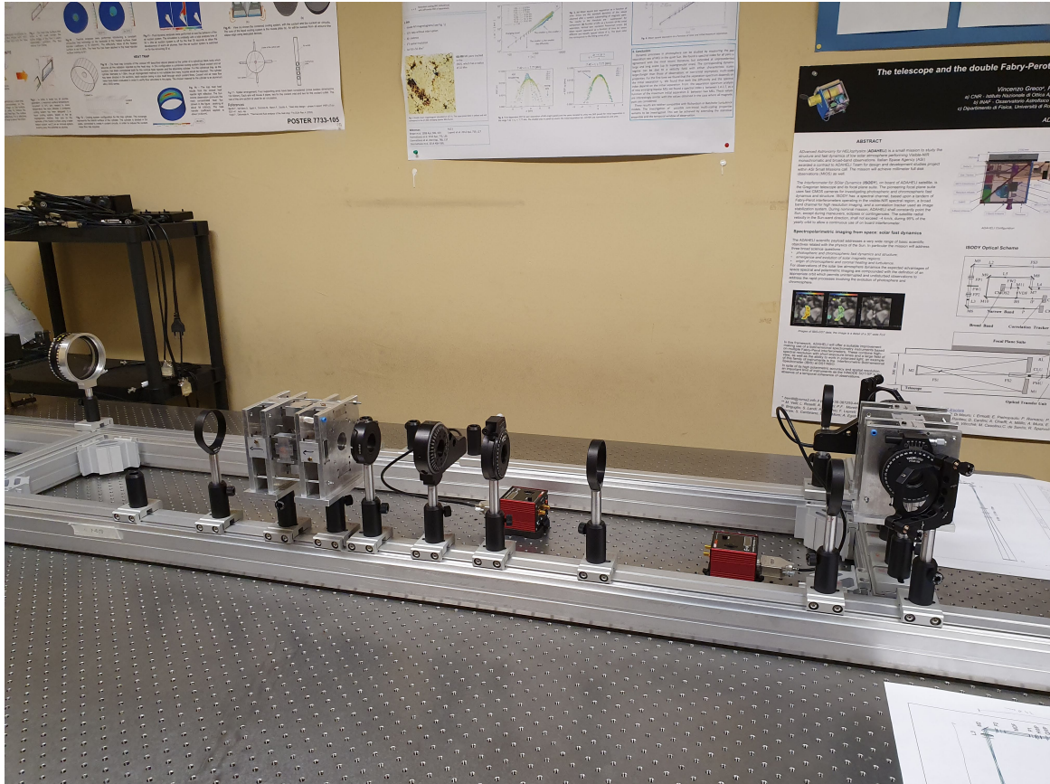
Figure 3.41: TSST MOF telescope in assembly phase. The holders and post-holders are placed on the optical rail. The next step is the insertion of the optical and polarimetric components.
