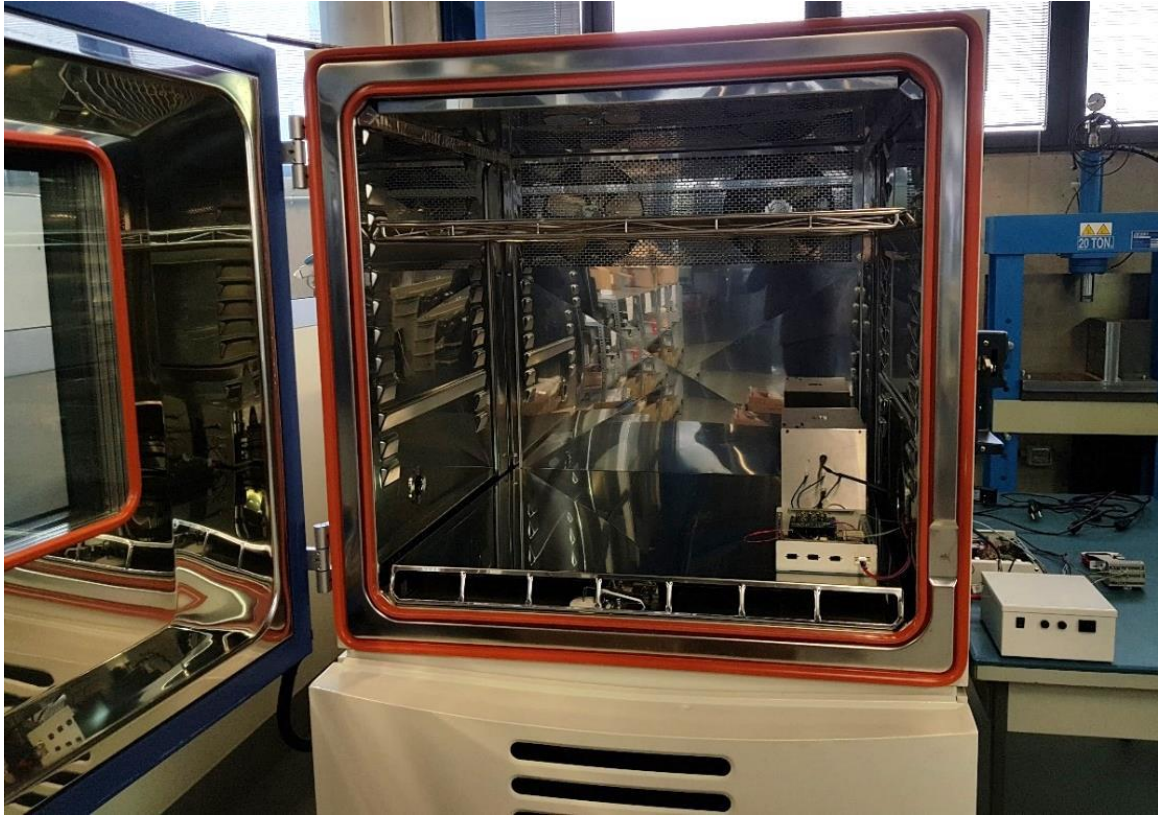
Figure 3.16: Climatic chamber by Weiss Technik with the GREST FPI 50 and the ADS100 inside. The power suppliers are placed outside.
