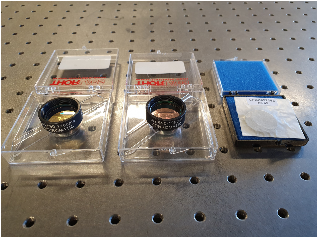
Figure 5.17: Quarter wave plate, half wave plate and linear polarizer of the MOF TSST telescope.
