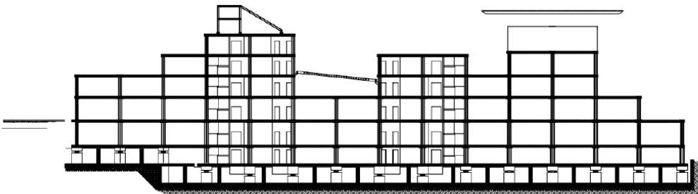
Fig. 13 Transversal section of the Lagonegro hospital building, with max dimension of 112m
