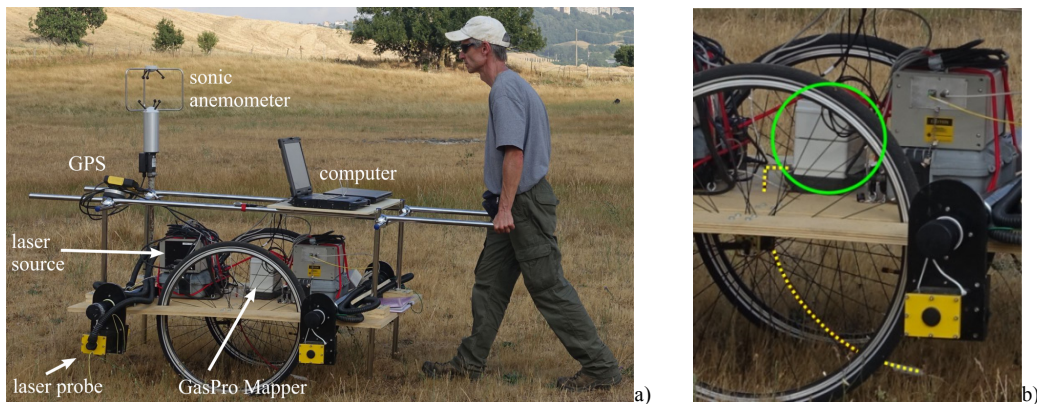
Figure 2. a) Cart with instruments mounted for spatial mapping. b) close-up of cart showing the Mapper system, with the pump, CO 2 sensor, batteries and electronics highlighted in the yellow circle and the sampling tube that is dragged below the cart shown by a dashed yellow line.
