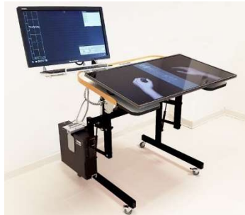
Figure 3: The Promotœr comprises a computer, a screen for the therapist feedback (EEG and EMG activity monitoring) and a screen for the ecological feedback to the patient (a virtual hand performing the imagined movement in successful trials). A commercial wireless EEG/EMG system (gTec, Austria) is used to record brain and muscular activity from the patient.
