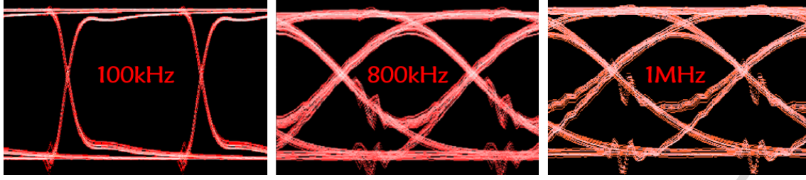
Figure 8. Eye-Diagram of the VLC channel realized with the CsFAMA-3 perovskite-based device, used as the photo-detector of the Rx (PVSK-PD + TIA).
