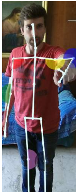
Figure 5.19. Pointing action performed by the user and recognized by the system. The pointed object is the camera itself.
