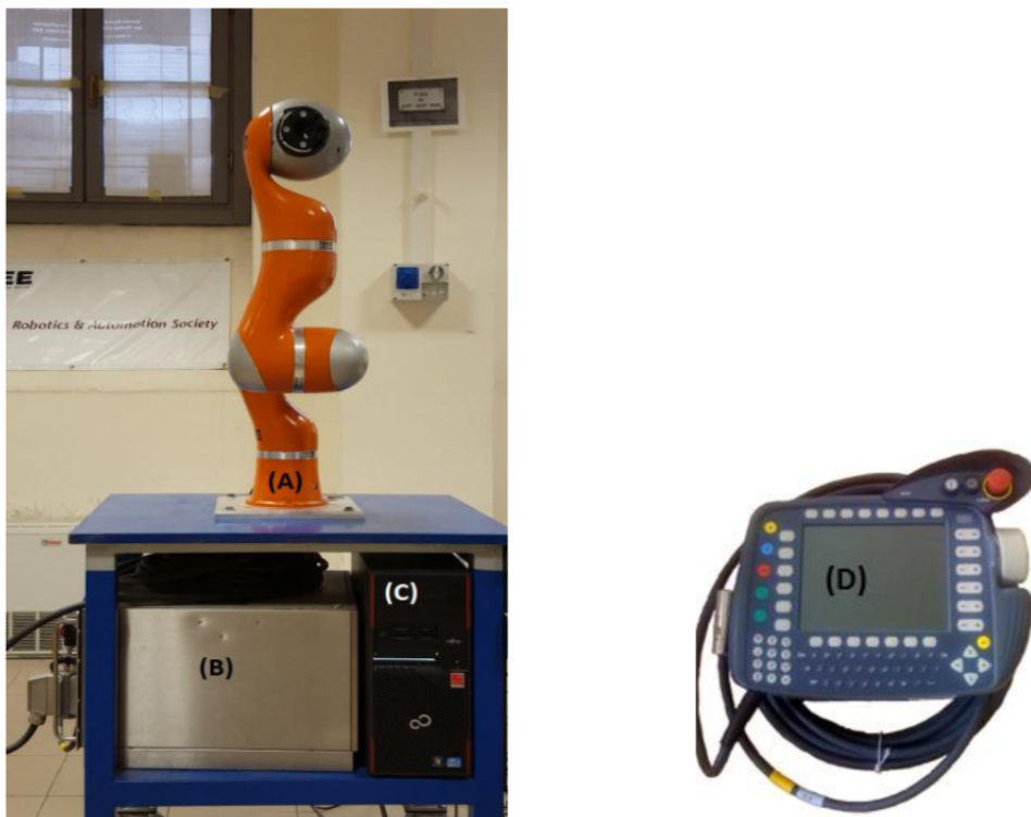
Figure B.2: The KUKA LWR system at DIAG Robotics Lab. (A) The LWR body. (B) The KR C2 lr robot controller unit. (C) PC node. (D) Kuka control panel.
