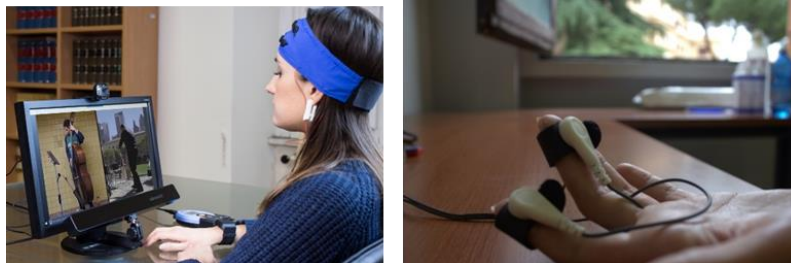
Figure 50 The image shows the recording session: the band 10 channel for EEG recordings on the left, the sensors for Autonomic data recording on the right.
