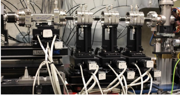
Figure 1: CBPM test-stand at FLASH1 with three undulator cBPMs (on the right) on remote movers [7].
