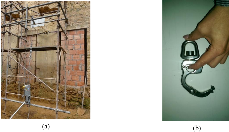
Figure 8 Snap shackle: connected to the wire rope (a); in opened position (b).
