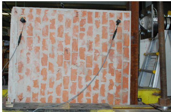
Figure 5: Shear tests on masonry panels with vertically aligned bed joints, laboratory test configuration.
