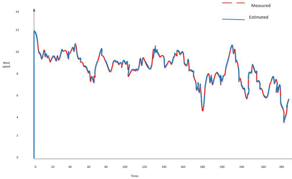
Figure 5.9: Wind speed estimation.
