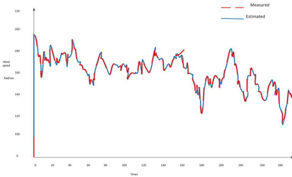
Figure 5.10: DFIG rotor speed estimation performance using AISE
