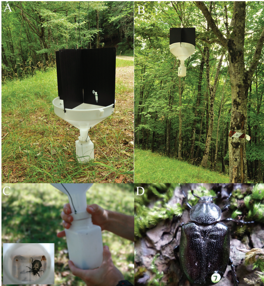
Figure 7. BCWT for capturing O. eremita . A Outline of a trap with an eppendorf vial containing the pheromone B positioning on tree branch C insertion of the funnel into the bottle, with details of hermit beetle captured by the trap (note the four small holes in the base to avoid water filling) D O. eremita with double marking procedure on elytra: dimples made by a small drill and a numbered sticker (photographs by E. Capogna: A–B , F. Bernardini: C , S. Chiari: D ).
