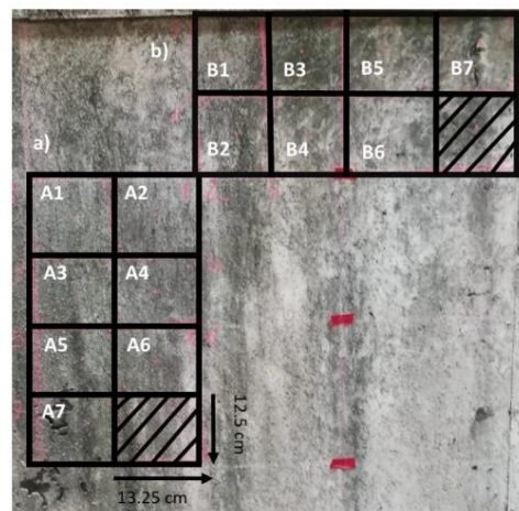
Fig. 1. The travertine biodegraded surface subjected to the cleaning procedures. a) Surfaces treated with the formulations containing the essential oils (A1 = O. vulgare ; A2 = O. vulgare + T. vulgaris ; A3 = T. vulgaris ; A4 = T. vulgaris + C. nepeta ; A5 = C. nepeta ; A6 = O. vulgare + C. nepeta ; A7 = O. vulgare + T. vulgaris + C. nepeta ). b) Surfaces treated with the formulations containing the terpene active components (B1 = carvacrol; B2 = carvacrol + thymol; B3 = thymol; B4 = thymol + pulegone; B5 = pulegone; B6 = carvacrol + pulegone; B7 = carvacrol + thymol + pulegone).
