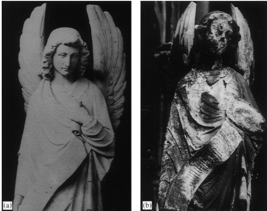
Figure 1 - Influence of biodeterioration processes on an angel statue at the “Peters”-Portal on the cathedral of Cologne (Germany); documented by the original object in 1880 ((a) photograph by Anselm Schmitz, Cologne) and the respective weathered statue in 1993 ((b) photograph by Dom1.2baumeister Prof. Dr. A. Wolff, Cologne)(Picture from Warsheid and Braams 2000 [1])
