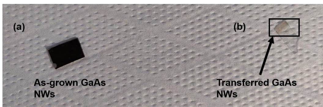
Figure 2. 8. The photographed images of (a) as-grown GaAs NW sample and (b) Mechanically transferred GaAs NWs onto a transparent quartz substrate for FTAS measurements.
